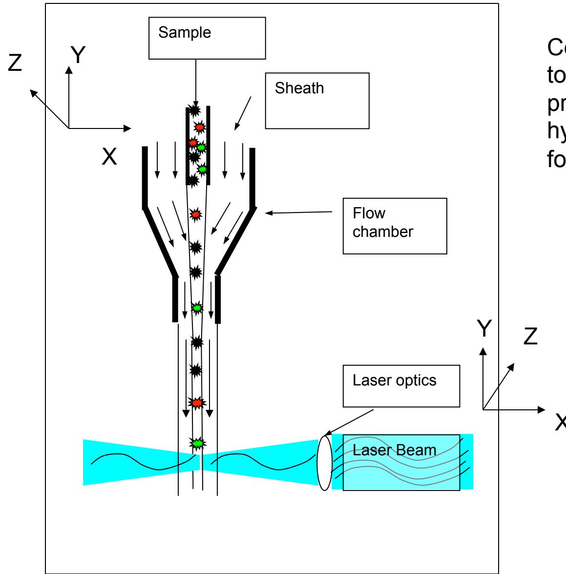
Cells are presented to the laser using principles of hydrodynamic focusing
