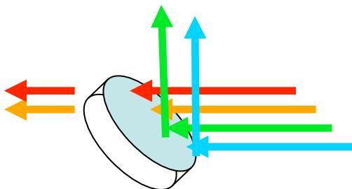
Dichroic Long Pass Optical Filter
