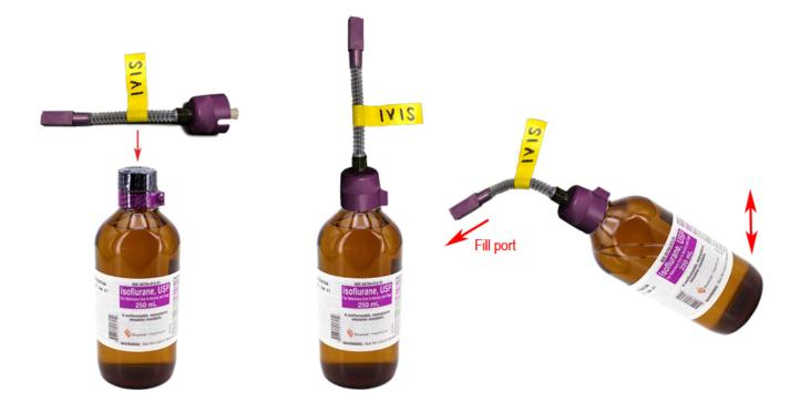
The CTAC provided filler tube should always be used to dispense your isoflurane into the vaporizer.
