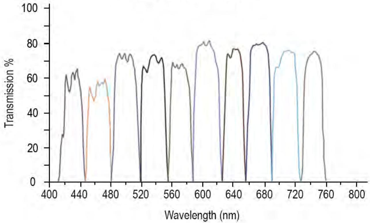
This image shows the different filter ranges for excitation on the IVIS Spectrum instrument. The covered wavelengths are from 410nm-760nm in 35nm increments
