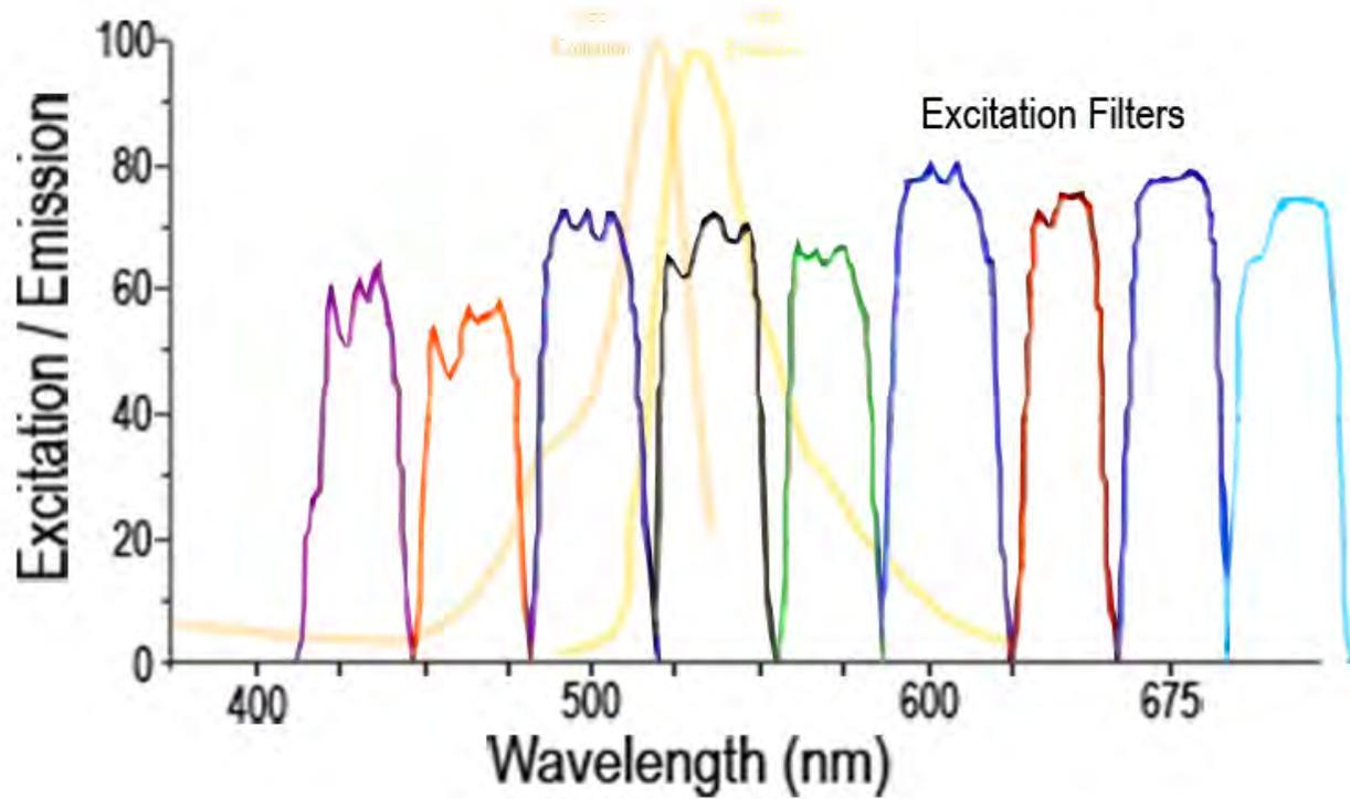
The two curves for YFP (Yellow Fluorescent Protein) are shown, the excitation curve is to the left of the emission curve. YFP is a challenging fluorophore to use, as its excitation and emission curves have a lot of overlap in their peak values. While there are 4 filters that cover the excitation curve, the first two are at the lower slope of the curve, the fourth is within the same range as the emission curve. The third filter on the left should be selected.
