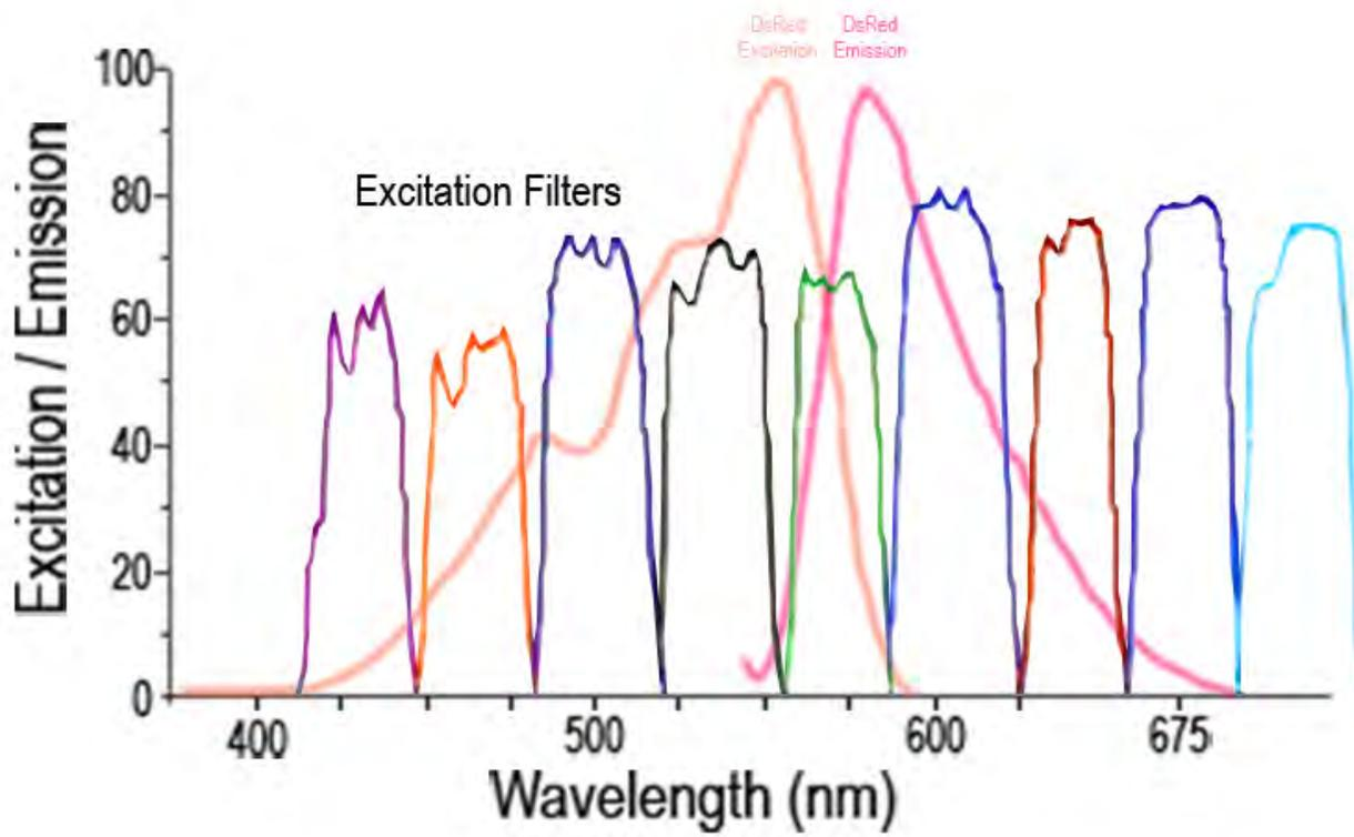
The two curves for DsRed (Discosoma Red Protein) are shown, the excitation curve is to the left of the emission curve. While there are 5 filters that cover the excitation curve, the first three are at the lower slope of the curve, the fifth is within the same range as the emission curve. The fourth filter on the left should be selected.
