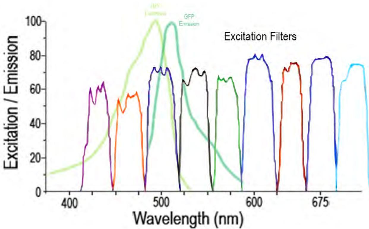
The two curves for GFP (Green Fluorescent Protein) are shown, the excitation curve is to the left of the emission curve. While there are 3 filters that cover the excitation curve, the first is at the lower slope of the curve, the third is within the same range as the emission curve. The second filter on the left should be selected.
