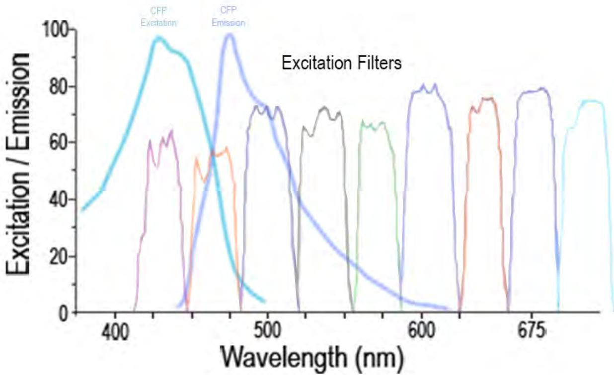
The two curves for CFP (Cyan Fluorescent Protein) are shown, the excitation curve is to the left of the emission curve. While there are 3 filters that cover the excitation curve, the second and third are within the same range as the emission curve. The first filter on the left should be selected.
