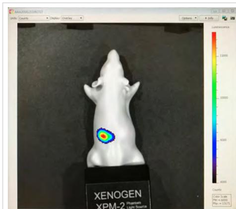
Same scan with the maximum gate value reduced to 6000 from an automatic value of 13171.
