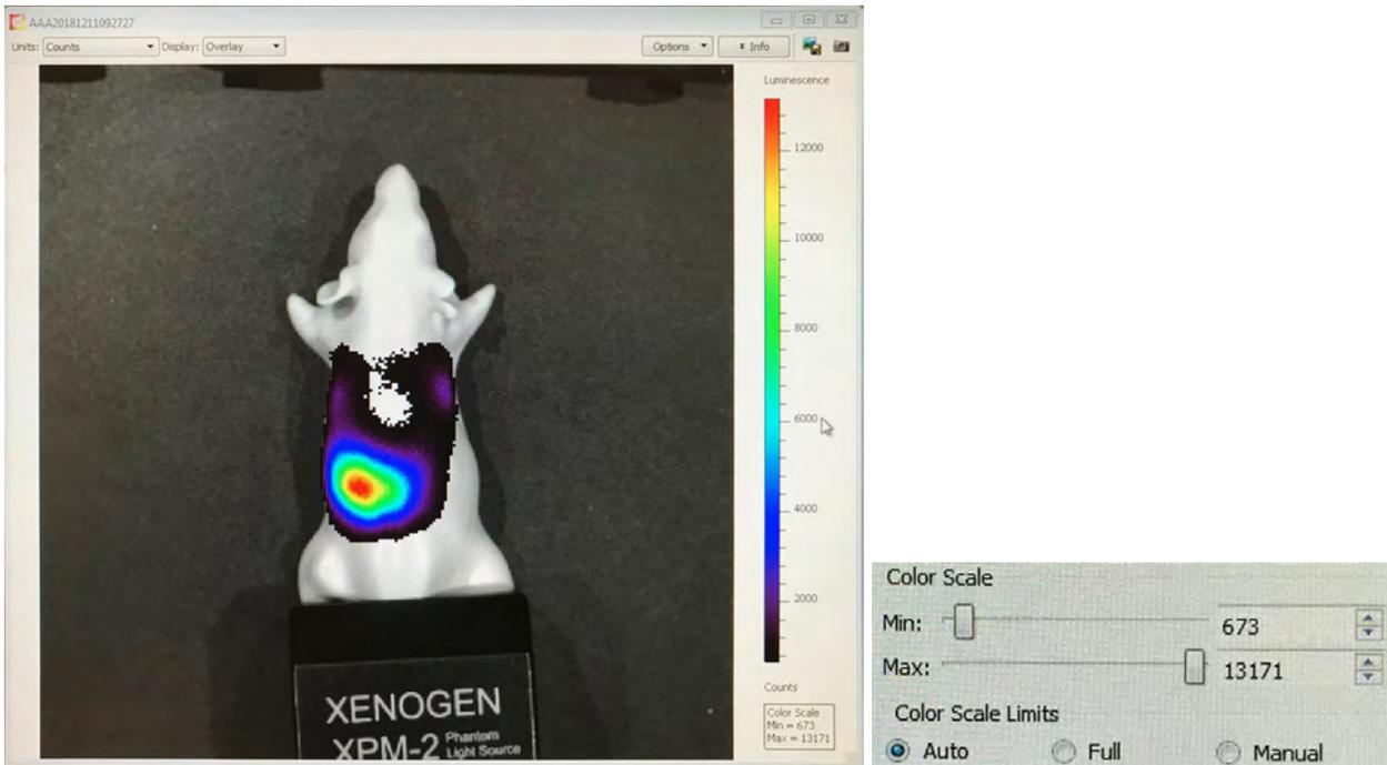
The IVIS software typically sets the gates at a minimum of 5% of signal and a maximum of 95% of signal.
