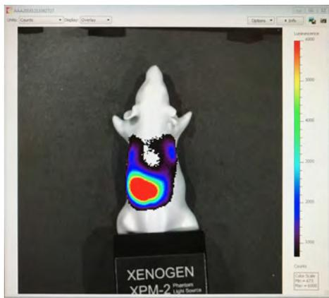
Same scan with the minimum gate value increased to 6000 from a automatic value of 13171.
