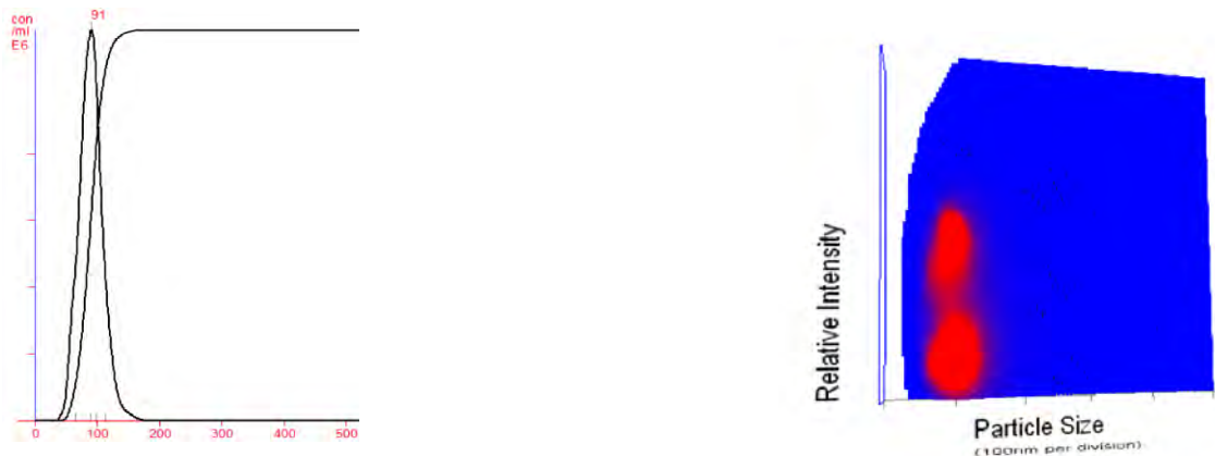
Figure 3: a) particle size distribution profile of a mixture of 92 nm polystyrene and 90 nm gold nanoparticles showing a single peak when measured by size alone; b) a 2D plot of the same mixture when size of each particle is plotted as a function of the amount of light it scatters allowing the much higher refractive index gold to be discriminated from the same sized polystyrene nanoparticles.
