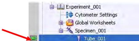
The current tube pointer indicates the tube to which instrument setting adjustments will apply and for which acquisition data will be shown.
